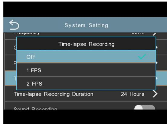
3.7 Time-lapse recording duration, The time can be set as 12 hours, 24 hours, 48 hours, 72 hours, Default 24 hours. (This function can only be used with a dedicated hardware kit, which can be purchased in stores)
